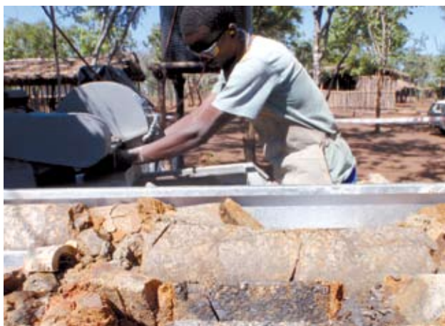
Core cutting underway at Massamba.
